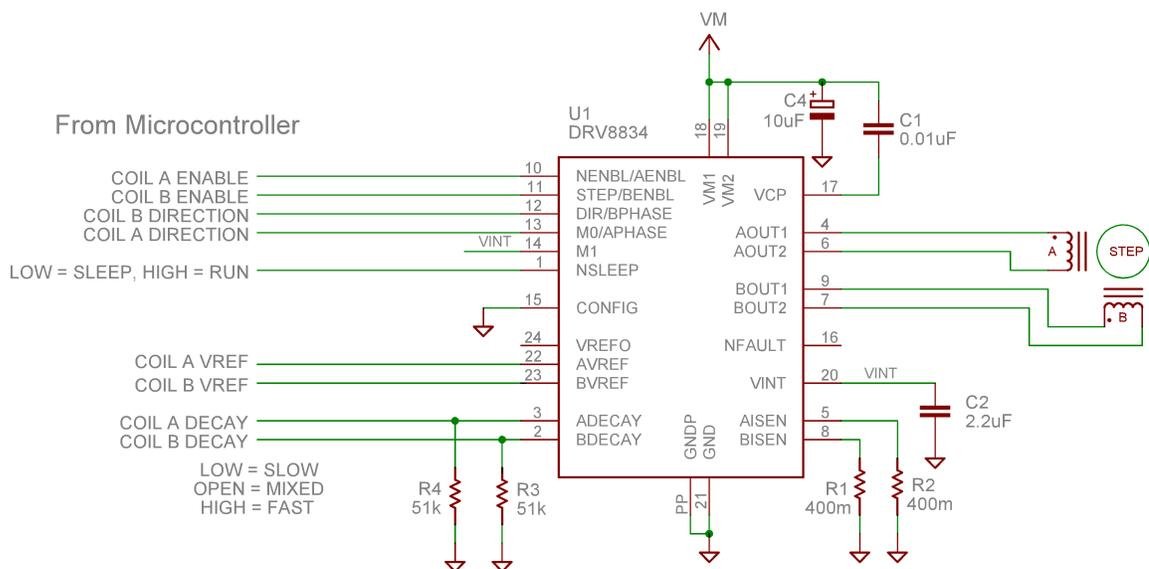
Figure 11. High-Resolution Microstepping
