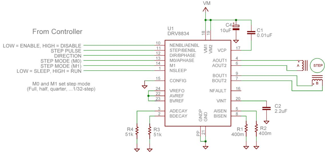
Figure 8. Indexer Mode Driving a Stepper Motor
