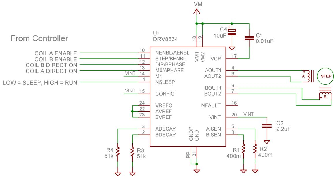
Figure 5. Phase/Enable Mode Driving a Stepper Motor
