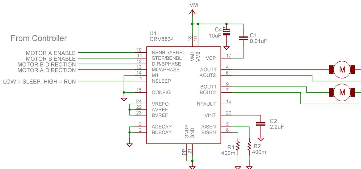
Figure 4. Phase/Enable Mode Driving Two DC Motors
